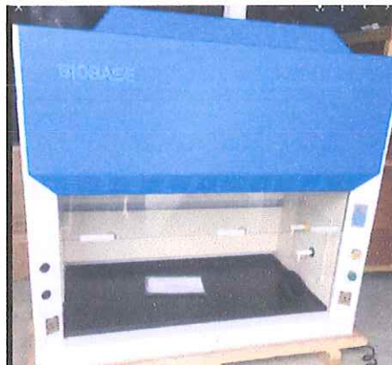
Figura 20: Campana extractora de gases
