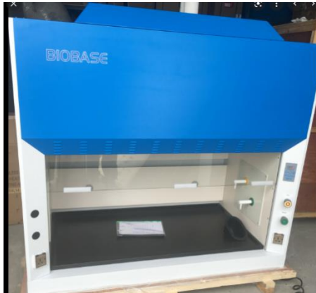
Figura 22: Campana extractora de gases
